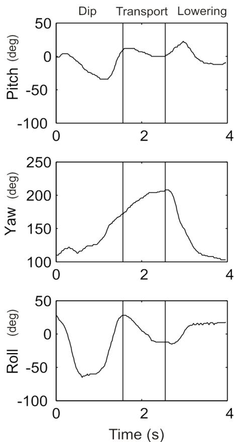
**Figure 5. Example output of pitch, roll and yaw angles from a movement at comfortable speed. Vertical lines mark automatically-detected transitions between phases of the eating cycle.**
