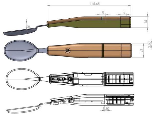
**Figure 6. Following feedback from professional caregivers, the spoon handle was re-designed, to be shorter and rounder.**
