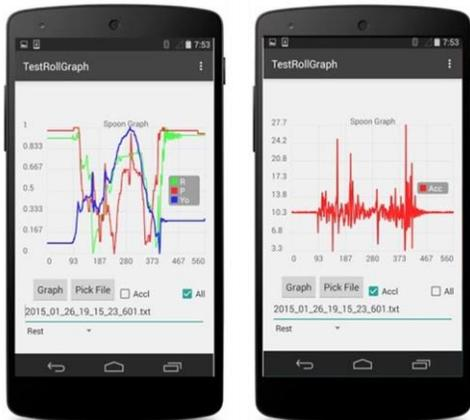
**Figure 3. Data is streamed from the spoon to an Android smartphone in real-time via Bluetooth. It is then classified and presented to the caregiver in a graph.**
