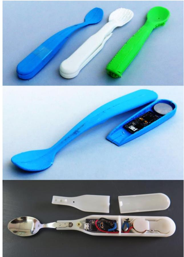
**Figure 2. Various form factors considered (and eventually rejected) during the iterative design process of DataSpoon.**
