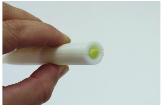
**Figure 7. An external switch was placed at the base of the handle in a recessed notch.**
